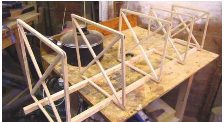
▲ Pic 3. A clamped-on fence helped to ensure that the notches for each shelf lined up accurately on the legs
